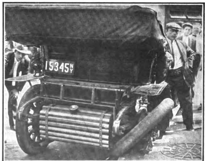
Fig. 2—Fiat skidded into gutter because of no non-skid device
